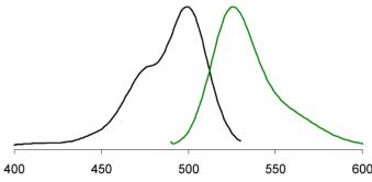
Excitation (left) and emission (right) spectra of Evagreen bound to dsDNA in PBS buffer (pH 7.3).
